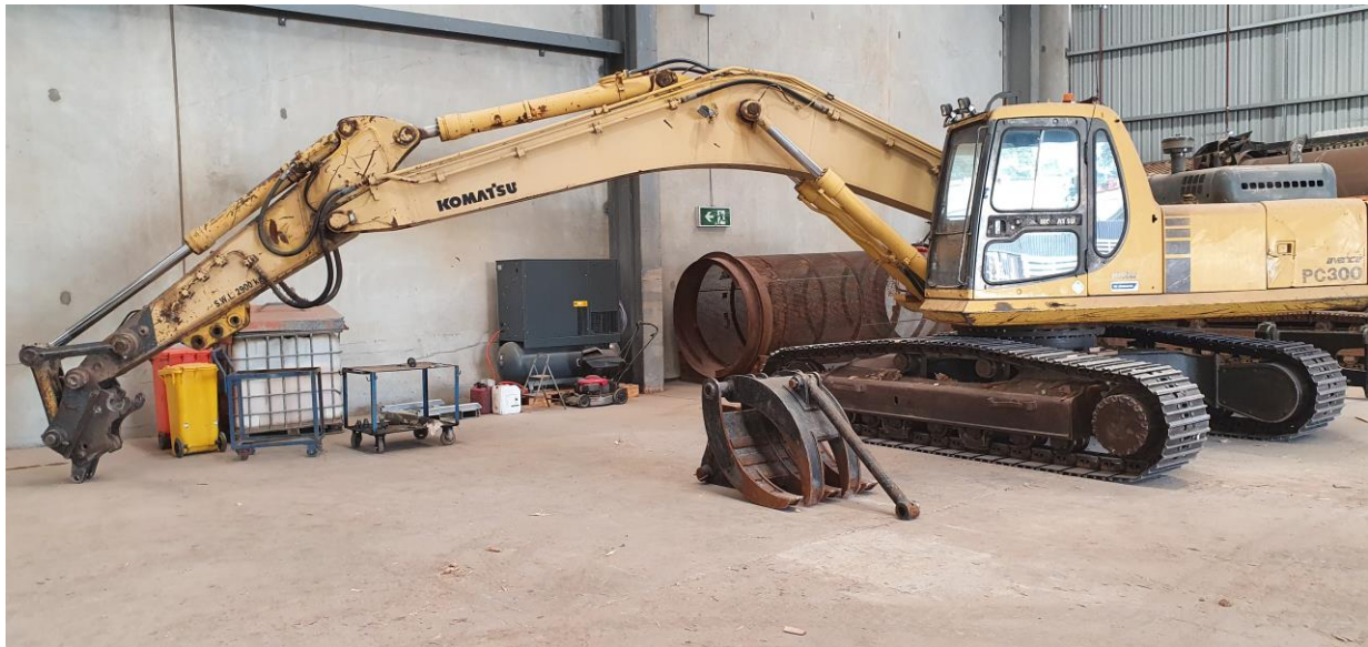
Figure 5 Typical excavator used for moving and minimising timbers
