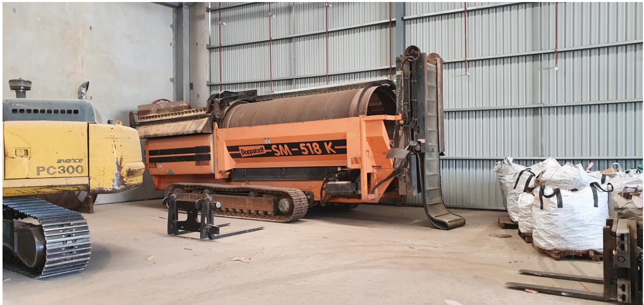
Figure 6 Typical Trommel used to separate different size of shredded materials.
